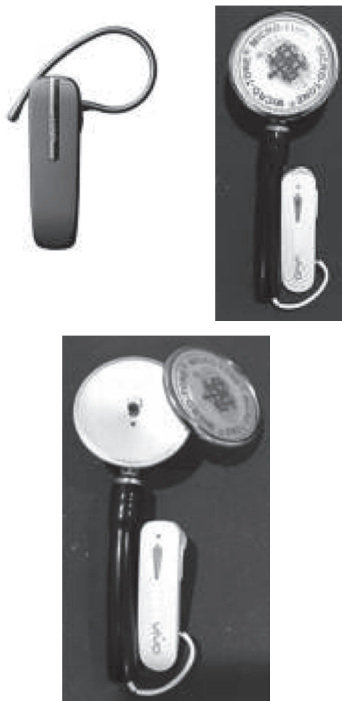
Fig.1. Assembling blue tooth stethoscope
