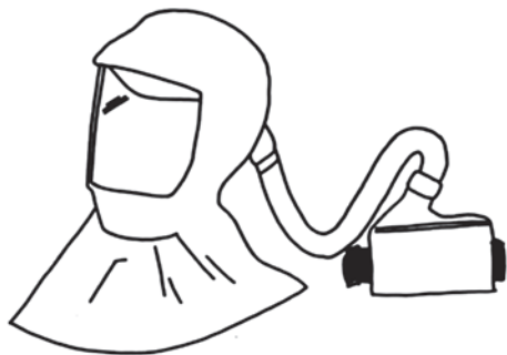
Fig.6. Example of a powered air purifying respirator (PAPR)
